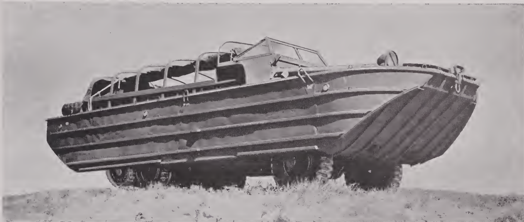
FIGURE 43. Front and side view of 1941 production DUKW, showing shape of bow.
